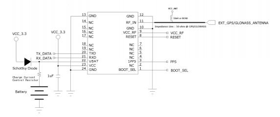
3. Example 1 for GPS/GLONASS Patch Antenna
