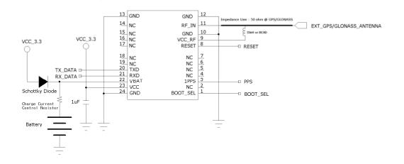
2. Example 2 for GPS/GLONASS External Active Antenna
